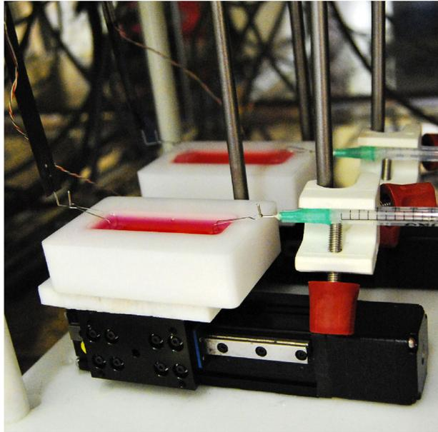
**Figure 1.** The tension culture force monitor (t-CFM). The collagen gels were cast and floated in medium in a mould positioned on a platform on a microprocessor-controlled stepping motor. The collagen gel was tethered between two floatation bars one is attached to a fixed point, whilst the other is attached to a force transducer.
