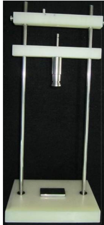
Fig. 1 Drop-mass press device for inflammation induction.
